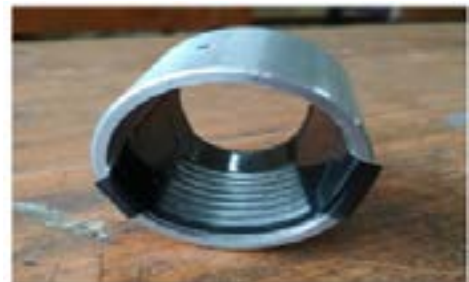
Figure 6: Radium maskant applied on the inner side of the bearing
