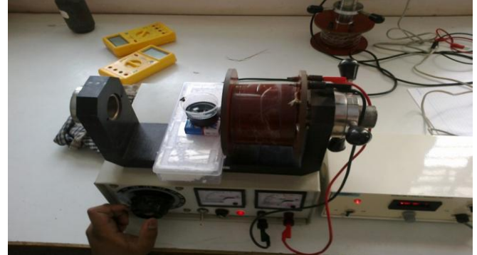
Fig. 1: Experimental set up for Magneto-Rheological Fluid characterization
