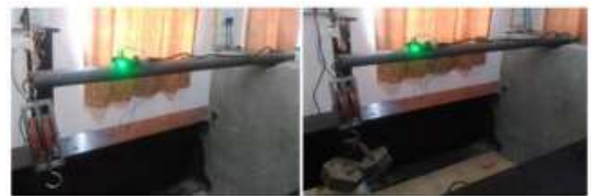
Figure 5 Composite blade in unloading and loading condition
