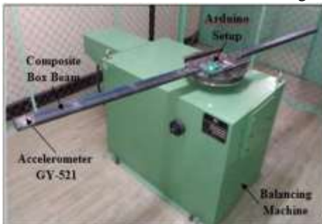
Figure 8 Experimental setup using GY-521 Accelerometer
